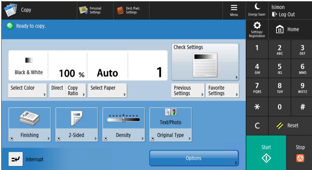
When you're done, be sure to hit Log Out at the top right of the screen (this will also happen automatically after roughly a minute of inactivity).
